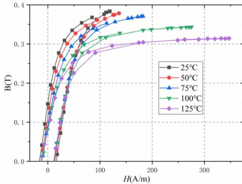
Figure 2: Hysteresis loops of ferrite at different temperatures
