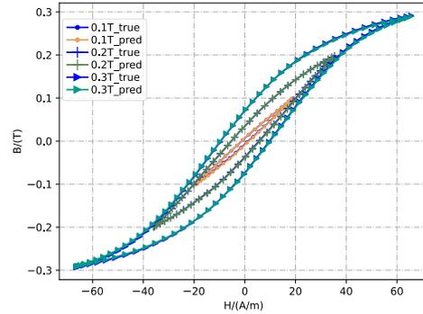
Figure 3: Model predicted value and experimental value of ferrite with different magnetic density at 100 °C
