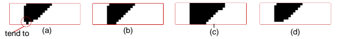
Fig. 5. (a) Deterministic optimized topology; (b) Robust optimized topology with L=0.5, \delta=1 ; (c) Distorted topology from (a) with L=0.5, \delta=1.5 ; (d) Robust optimized topology with L=0.5, \delta=1.5
